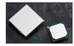
Silver-Filled Polyurethane Conductive Coating for EMI Shielding
