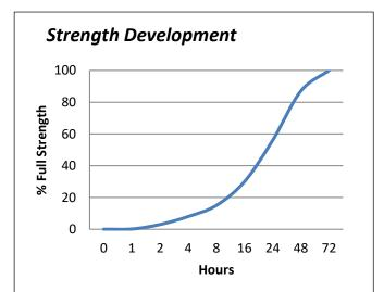
Graph shows typical strength development of bonded components at 23°C. Curing at higher or lower temperatures may affect cure speed.
