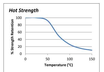
"Hot strength" shear strength tests performed on mild steel. Fully cured specimens conditioned to pull temperature for 30 minutes before testing at temperature. ET5383 can withstand higher temperatures for brief periods (such as for paint baking and wave soldering processes) providing the joint is not unduly stressed. The minimum temperature the cured adhesive can be exposed to is -40°C (-40°F) depending on the materials being bonded.
