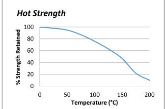
"Hot strength" shear strength tests performed on mild steel. Fully cured specimens conditioned to pull temperature for 30 minutes before testing at temperature. TA4592 can withstand higher temperatures for brief periods (such as for paint baking and wave soldering processes) providing the joint is not unduly stressed. The minimum temperature the cured adhesive can be exposed to is -55°C (-65°F) depending on the materials being bonded.
